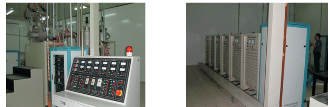
图 1 等离子体蒸发纳米金属粉体连续制备生产线图片 continuous metal nano-powder production line of plasma evaporation
